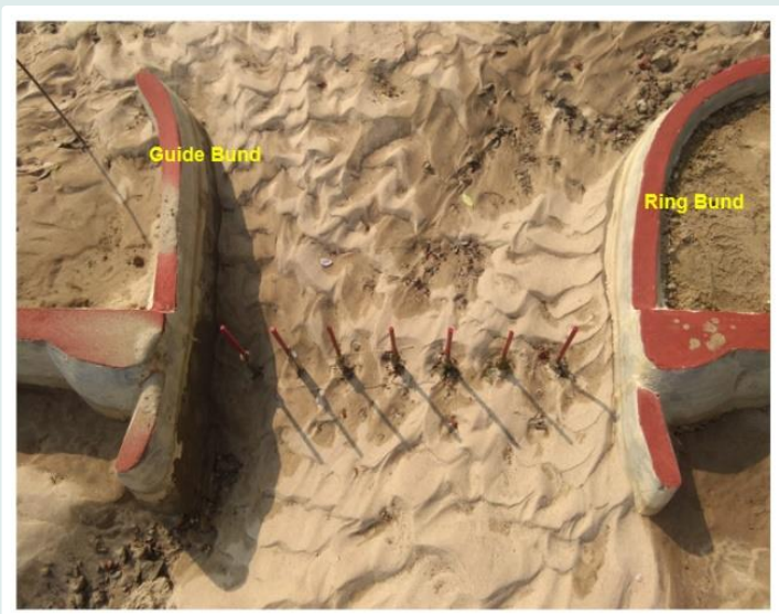
River Bed Condition in the Bridge on Bhuthi Balan River at Design Discharge with Guide and Ring Bunds
