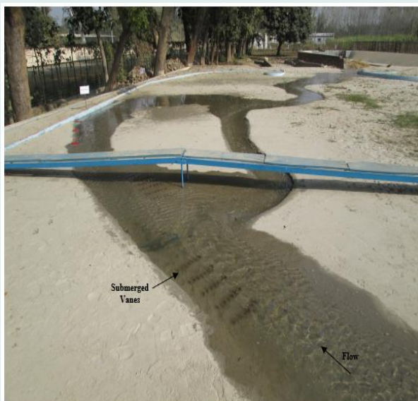
Submerged Vanes and RCC Jack Jetties under running condition
