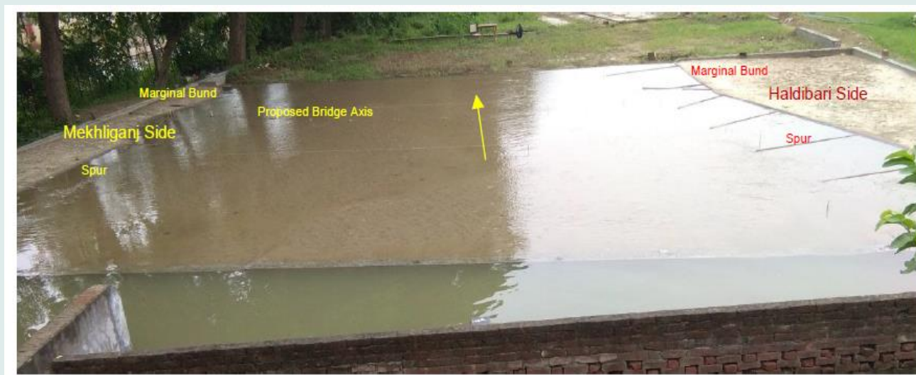
General View of the Model without Bridge from Upstream at 21,600 cumec discharge
