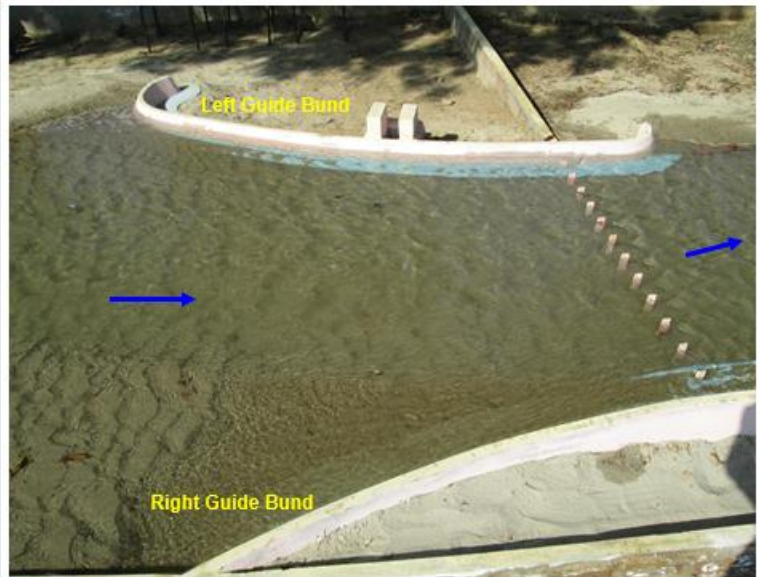
Flow Condition at Left Guide Bund – Design Discharge
