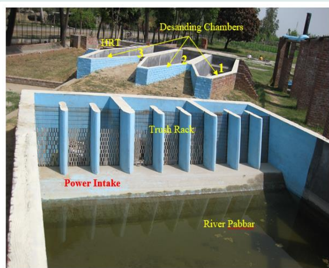
Another View of De-sanding Chamber Physical Model
