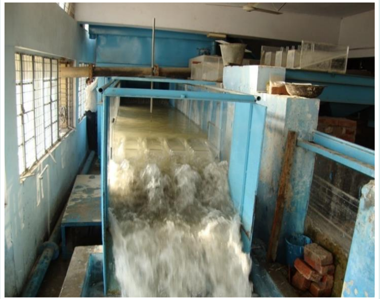
Running view of Model at 1128 m 3 / Sec discharge
