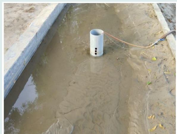
Water Intake Structure 20 m away from the Bank
